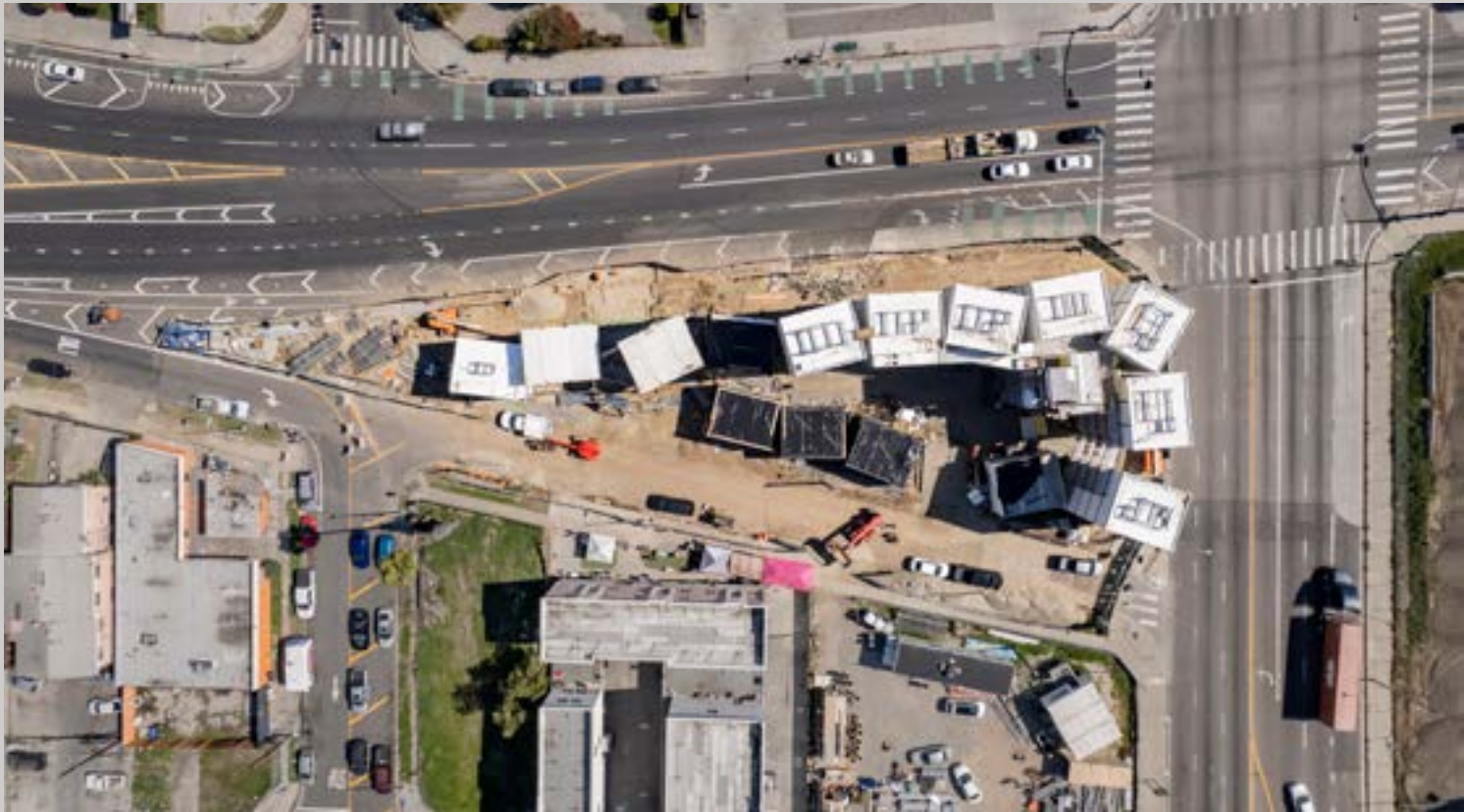
Modules are arranged to shield units and the interior circulation spaces from the nearby freeway. (Paul Vu, courtesy LOHA)
