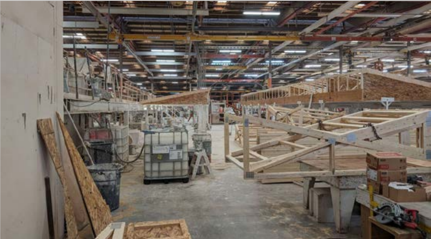
CrossMods™ being assembled for NPHS in Southern California. (Courtesy NPHS)
